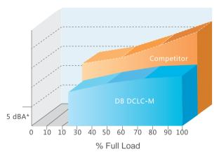
The rotating impeller and shaft is levitated at the magnetic field cushion, and have no physical contact with other components during the operation. Therefore, the unit structural vibration is virtually zero. With the permanent magnet DC brushless motor, the noise level is further reduced. Dunham-Bush DCLC-M centrifugal chillers will be best solution for installation at sound level sensitive area.
