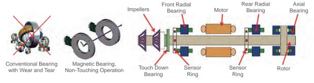
The axially and radially located magnetic bearings create electromagnetic field which levitates the shaft during rotation and float on the magnetic cushion. This has prevented contact between compressor shaft and other metallic surfaces, and thus, the oil lubrication system is no longer needed. The proximity sensors at bearings sense rotor movements and adjustment are made accordingly in the rate of 6,000,000 times per minute. This ensures presicion of rotor position in the magnetic field.
