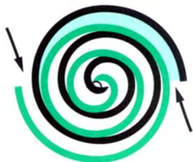
Compression in the scroll is created by the interaction of an orbiting spiral and a stationary spiral. Gas enters the outer openings as one of the spirals orbits.
