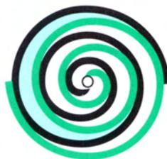
The open passages are sealed off as gas is drawn into the spiral.
