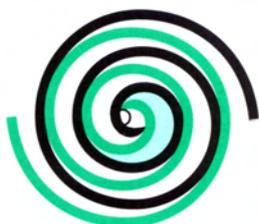
Actually, during operation, all six gas passages are in various stages of compression at all times, resulting in nearly continuous suction and discharge.
