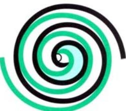
Actually, during operation, all six gas passages are in various stages of compression at all times, resulting in nearly continuous suction and discharge.
